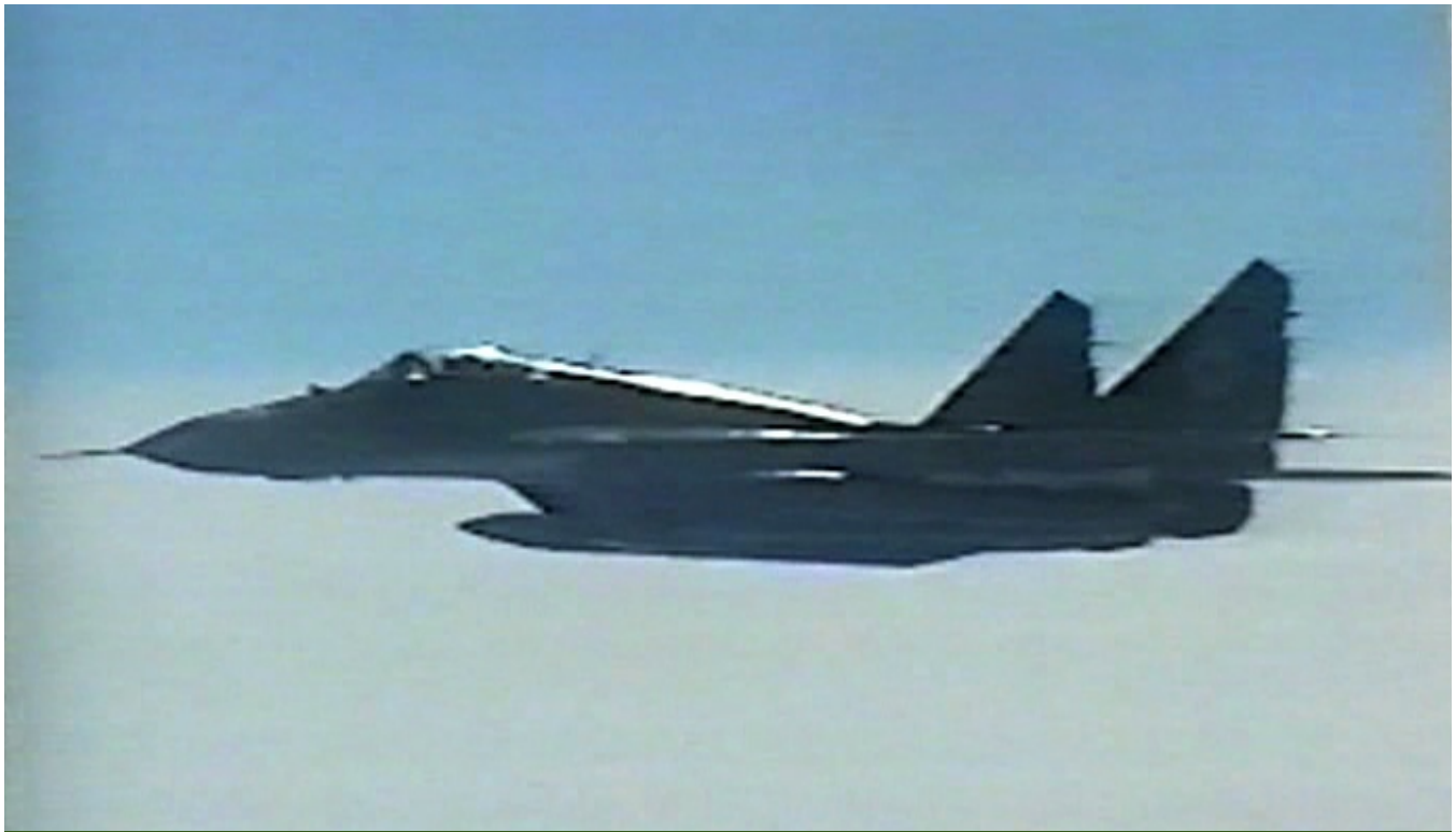
One of the two KPAF MiG-29 keeping station on the starboard side of the USAF RC-135S COBRA BALL on March 2, 2003. Just visible in this image is the IRST and ODD RODS antennas in front of the canopy. Note the slight "hump" behind the canopy suggestive of the FULCRUM C, although this could be distorted by camera angle and lighting. (USAF)
