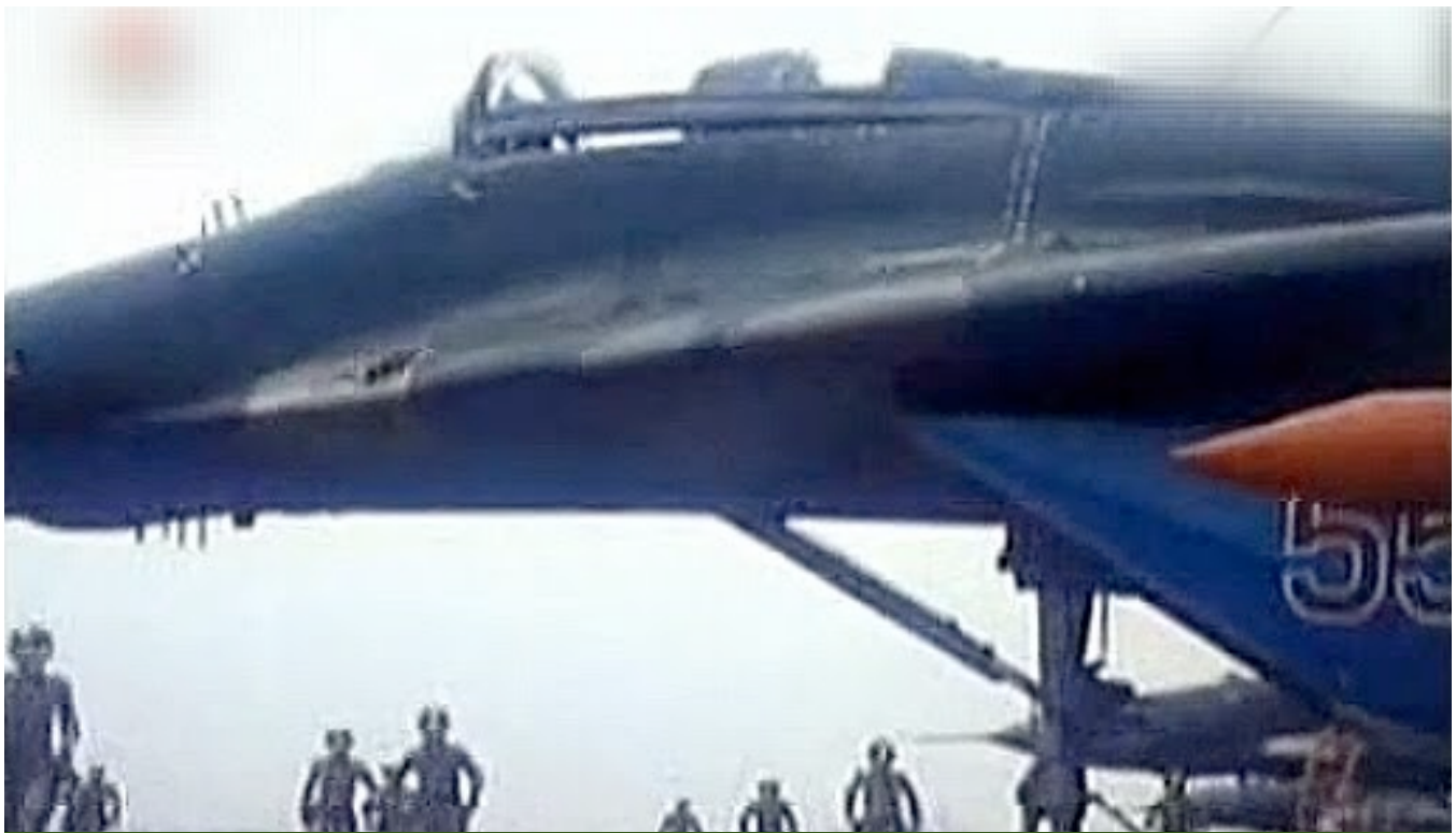
A closeup of the starboard side of MiG-29B #55X. Visible are the ODD RODS antennas in front of the canopy, the gun port in the port wing root and the tip of what appears to be a R-27 AA-10C ALAMO under the port wing. (KPAF via http://elhangardetj.blogspot.com/2011/02/mig-29-de-corea-del-norte.html )
