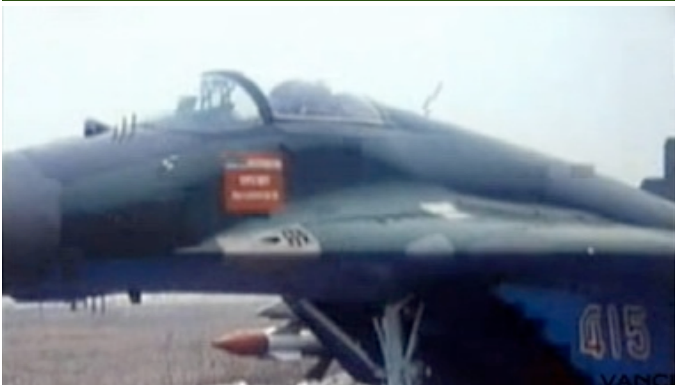
A closeup of the starboard side of MiG-29B #415. Note theIRST and ODD RODS antennas in front of the canopy, the commemorative placard below the canopy, the gun port in the port wing root and the tip of what appears to be a R-27 AA-10C ALAMO under the starboard wing. (KPAF via http://elhangardetj.blogspot.com/2011/02/mig-29-de-corea-del-norte.html )
