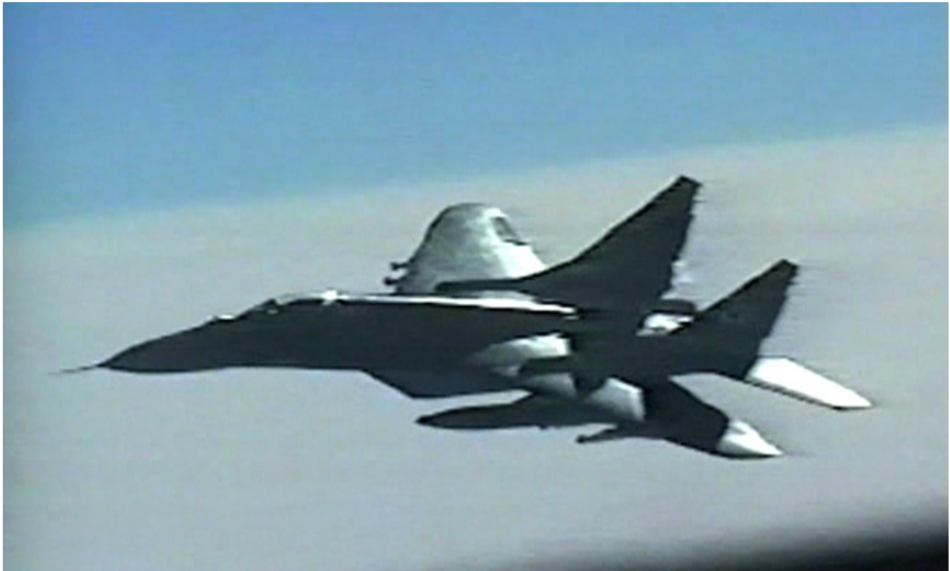
One of the two KPAF MiG-29s that intercepted a USAF RC-135S COBRA BALL on March 2, 2003. Visible in this image are the port drop tank on the inner pylon and what appear to be R-60 AA-8 APHID AAMs on the outer two pylons. This image was captured from a video taken by one of the crew members aboard the RC-135S. (USAF)
