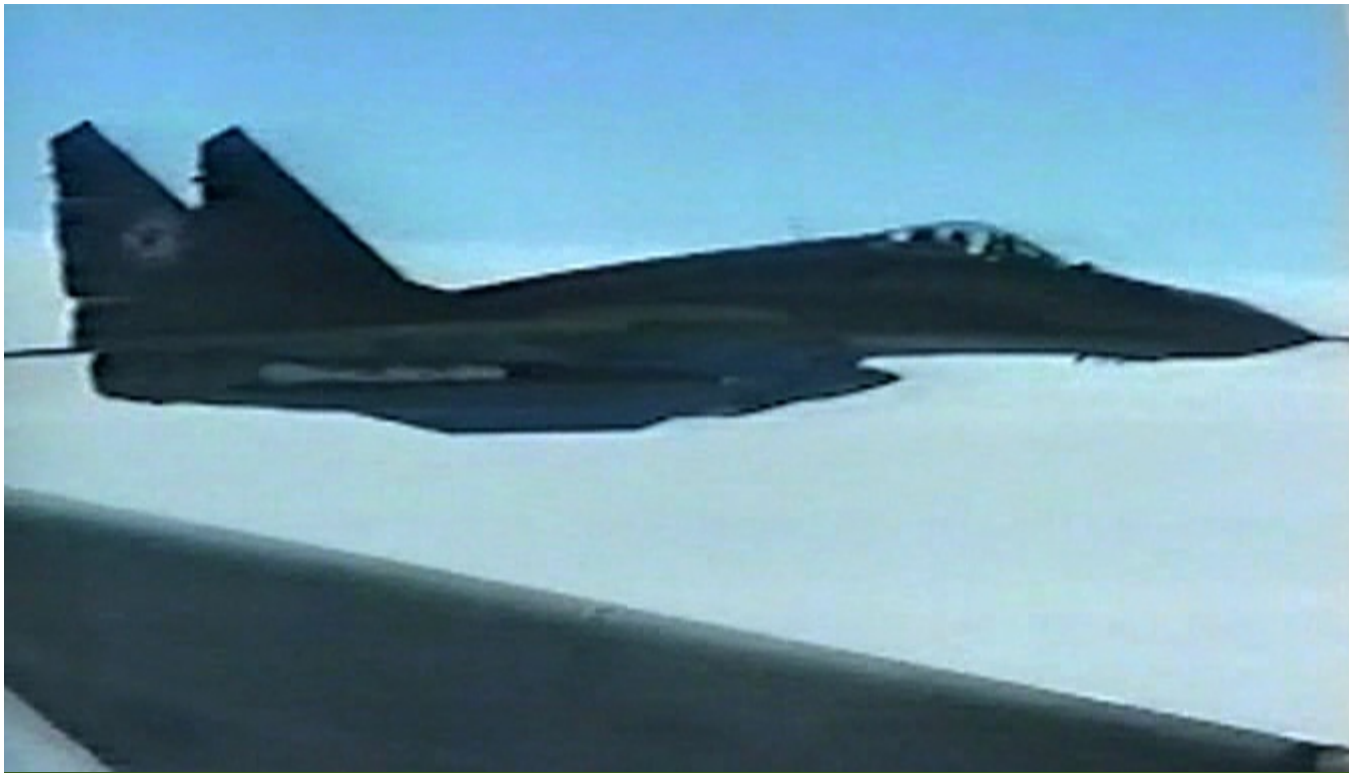
One of the MiG-29s keeping station on the port side of the USAF RC-135S COBRA BALL on March 2, 2003. Visible in this image are the starboard drop tank on the inner pylon and what appear to be R-60 AA-8 APHID AAMs on the outer pylons. The ODD RODS antenna and IRST are just visible in front of the canopy. (USAF)
